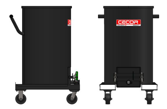
CECOR'S HEAVY DUTY 55-GALLON DRUM TANK, MADE OF HEAVY GAUGE STEEL, IS STRONGER THAN A STANDARD 55-GALLON DRUM. THE TANK IS MOUNTED ON FOUR CASTERS FOR EASY ROLLING AND MANEUVERABILITY. FORK POCKETS BUILT INTO THE BASE PROVIDE EASY HANDLING BY FORK TRUCK. THE TANK FEATURES AN 8" X 10" CLEANOUT DOOR FOR REMOVING SETTLED SOLIDS. VALVE IN DOOR PERMITS FLUID TO DRAIN OUT, LEAVING THE SOLIDS.
