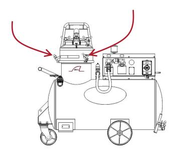
3. LIFT FILTER OUT OF SUMP CLEANER TANK USING HOIST OR FORKLIFT. CAUTION: KEEP HANDS AND FINGERS CLEAR OF POT OPENING IN SUMP CLEANER WHEN REMOVING FILTER!
