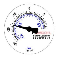
5. TURN SWITCH OFF. THE NEGATIVE PRESSURE IN THE TANK WILL CAUSE THE PUMP TO ROTATE BACKWARDS UNTIL THE PRESSURE EQUALIZES.
