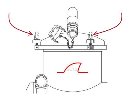
3. REMOVE FILTER. USE THE SIDES OF THE COARSE AND FINE FILTERS TO LIFT. FOR POLY FILTER, USE THE HANDLES ON SIDES AND BOTTOM TO REMOVE.
