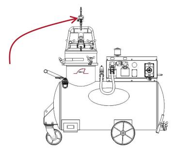
4. POSITION FILTER ABOVE CONTAINER INTO WHICH THE SLUDGE IS TO BE EMPTIED. DISTANCE BETWEEN BOTTOM OF FILTER AND CONTAINER BOTTOM OR "D" DIMENSION, SHOWN IN FIGURE BELOW, AND SHOULD BE APPROXIMATELY 2 TO 3 FEET ON F23 TO PREVENT DAMAGE TO FILTER SLEEVE WHEN DUMPED. DRAINING FILTER BEFORE POSITIONING AND USING A CONTAINER WITH A DRY BOTTOM AND SUITABLE CAPACITY WILL HELP REDUCE POSSIBLE FILTER SPLASH BACK.
