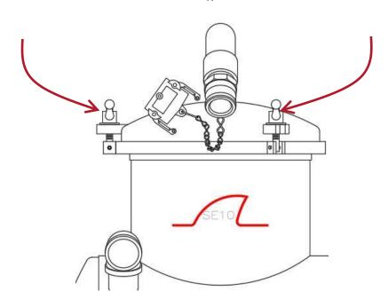
5. WITH UNIT IN SUCTION MODE AND POT LID CAPPED, TURN UNIT ON AND TO TIGHTEN WING NUTS. THIS PROVIDES EQUAL PRESSURE ON THE POT LID GASKET CREATING BEST SEAL.
