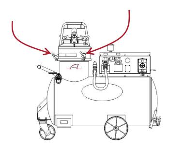
3. LIFT FILTER OUT OF SUMP CLEANER TANK USING HOIST OR FORKLIFT. CAUTION: KEEP HANDS AND FINGERS CLEAR OF POT OPENING IN SUMP CLEANER WHEN REMOVING FILTER!
