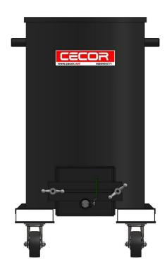
CECOR'S HEAVY DUTY 55-GALLON DRUM TANK, MADE OF HEAVY GAUGE STEEL, IS STRONGER THAN A STANDARD 55-GALLON DRUM. THE TANK IS MOUNTED ON FOUR CASTERS FOR EASY ROLLING AND MANEUVERABILITY. FORK POCKETS BUILT INTO THE BASE PROVIDE EASY HANDLING BY FORK TRUCK. THE TANK FEATURES AN 8" X 10" CLEANOUT DOOR FOR REMOVING SETTLED SOLIDS. VALVE IN DOOR PERMITS FLUID TO DRAIN OUT, LEAVING THE SOLIDS.
